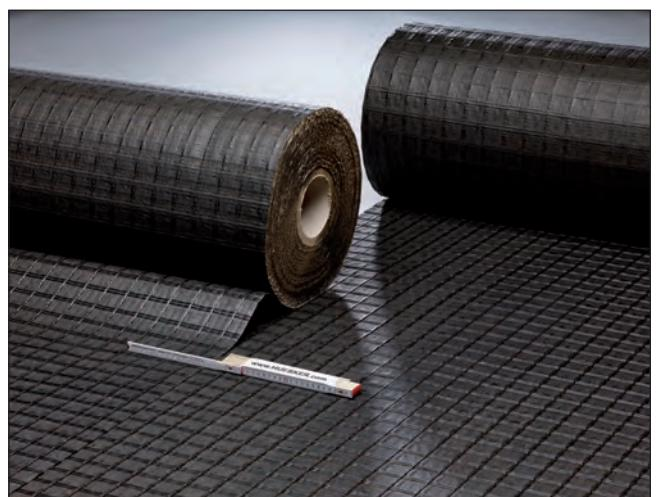
The end of a roll should always be placed over the beginning of the next, ensuring the overlap is not lifted during the asphalt covering operation.
