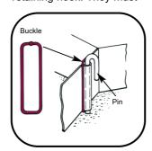
be sized to provide adequate anchorage under site conditions. Pin layout depends on slope angle (our design guide can be found at www.colbondgeosynthetics.com). The buckles are supplied by Colbond in packs of 300.
