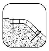
The panel is tensioned manually and fixed temporarily at the toe to prevent uneven deformation during filling. The buckles connecting adjacent panels should be placed where the cell walls are double layer. They transfer loads induced in the respective cells further down the slope.
